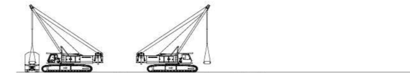
Unloading and assembling of central counterweight plate
